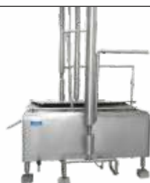
Chilled Water Tank
